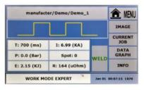
This system is recommended especially for HSS which will be widely used in future car models. The use is extremely easy by means of a touch-screen display offering the choice of manual, automatic or specific programs of the car manufacturers. By means of a USB flash memory, it is also possible to upload new welding programs or send to a PC the results of the welding process for a further elaboration.
